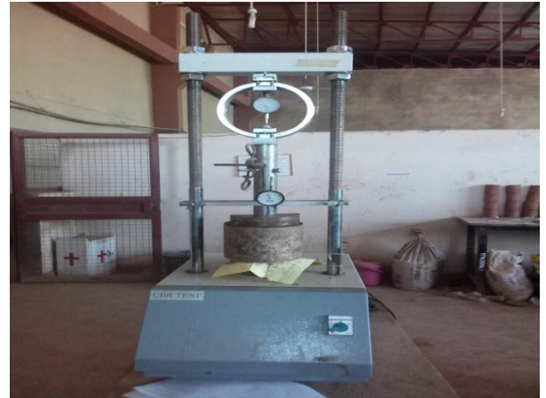
Plate II: California Bearing Ratio test of samples
