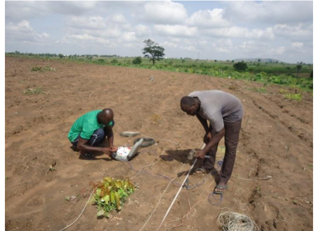
Figure 5: 2D Electrical Resistivity Data acquisition
