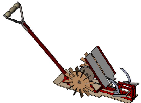
Figure 2: Isometric Drawing of the Designed Manually Operated Rice Transplanter
