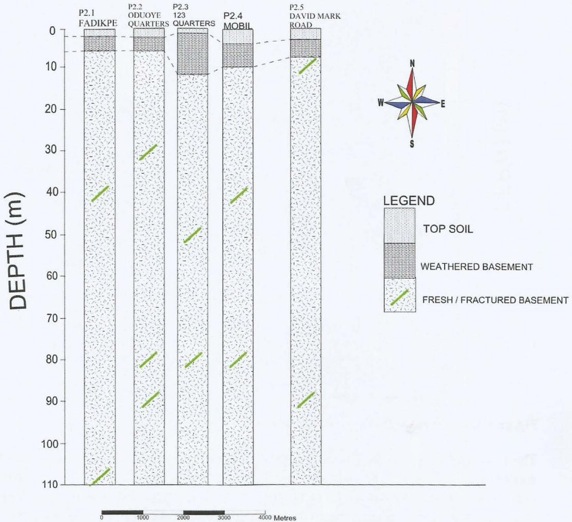
Figure 8: Geoelectric logs of points along profile 2
