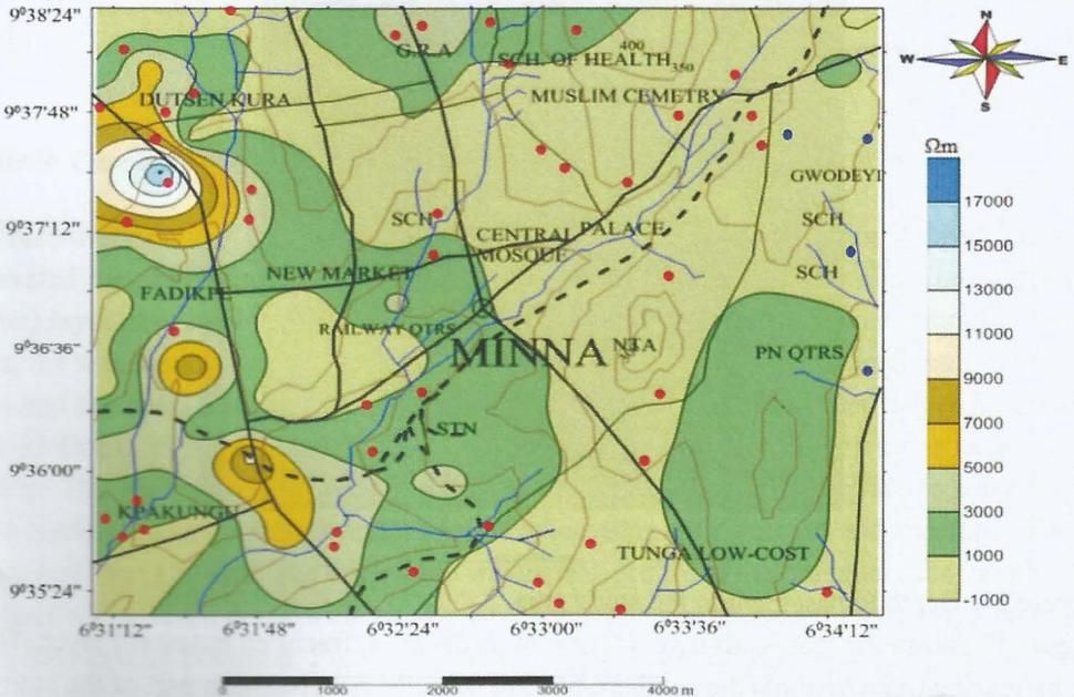
Figure 13: Relationship between geology and resistivity within the study area. Blue and red dots represent schist and granite rocks respectively.
