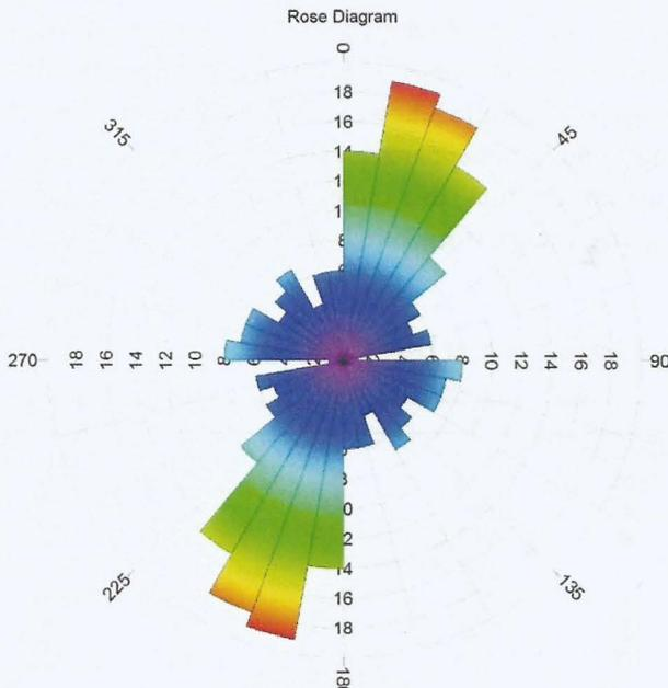
Figure 3: Rosette diagram of joint directions
