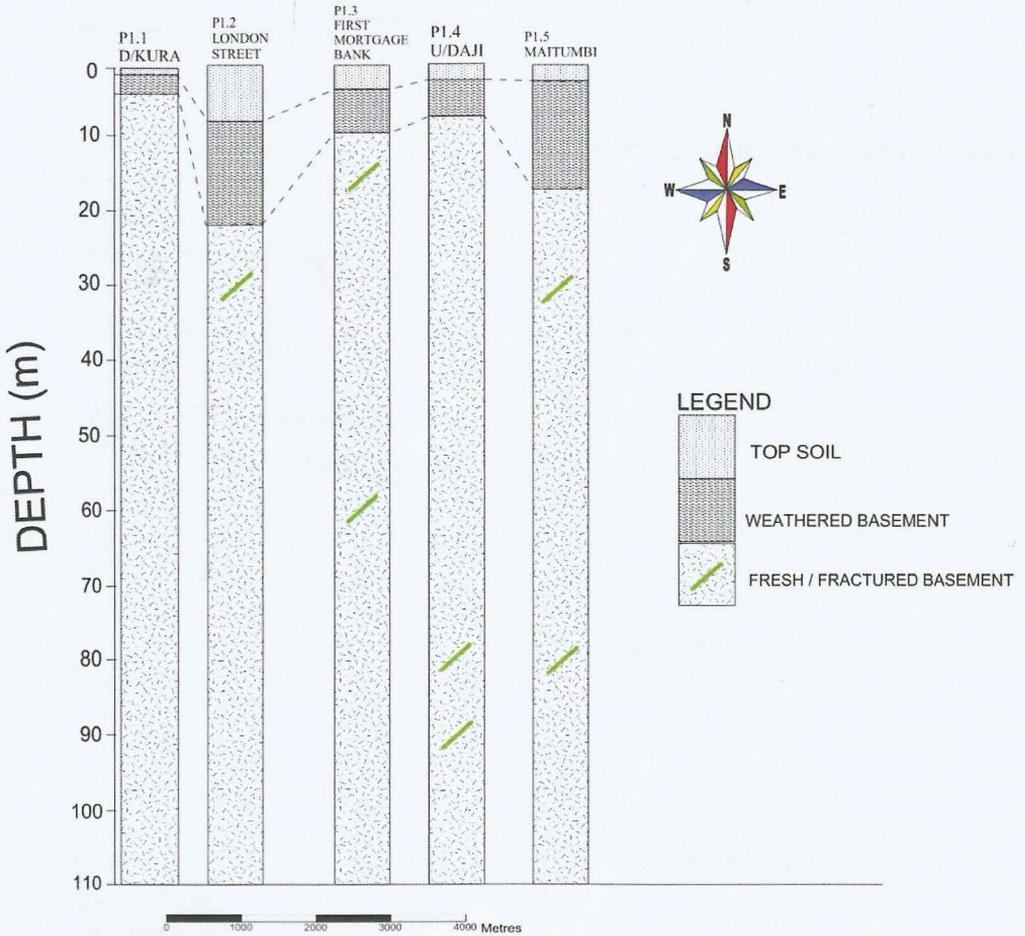
Figure 7: Geoelectric logs of points along profile 1
