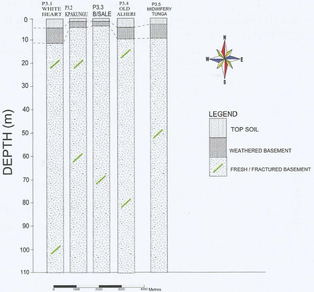
Figure 9: Geoelectric logs of points along profile 3
