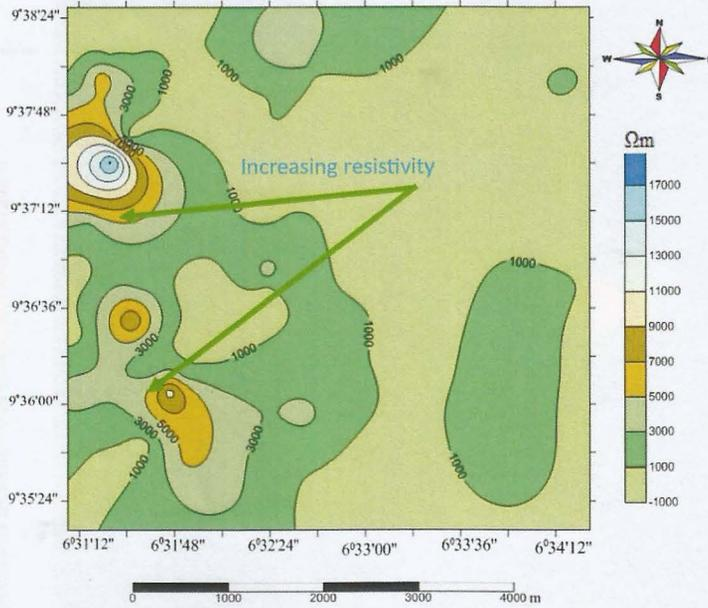
Figure 12: Isoresistivity plot of fresh/fractured basement layer
