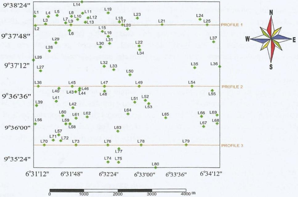
Figure 1: Horizontal Electrical Profiling and Vertical Electrical Sounding points
