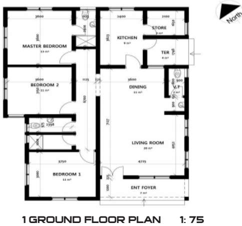
Figure 3 (Type 1): Typical floor plan of a single family bungalow housing in the study area.
