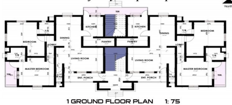
Figure 6 (Type 3): Typical ground floor plan of a two families' semidetached storey housing unit in the study area.
