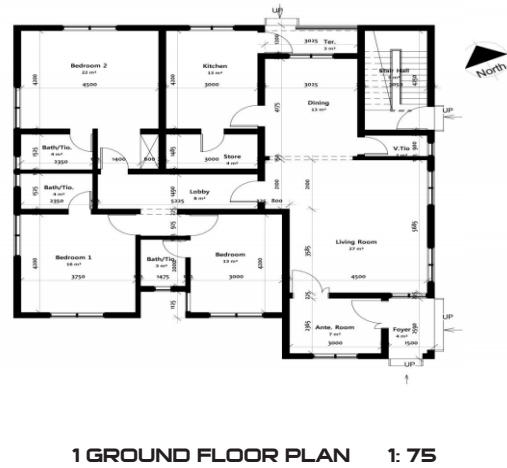
Figure 4 (Type 2): Typical Ground floor plan of a single storey family housing unit in the study area.
