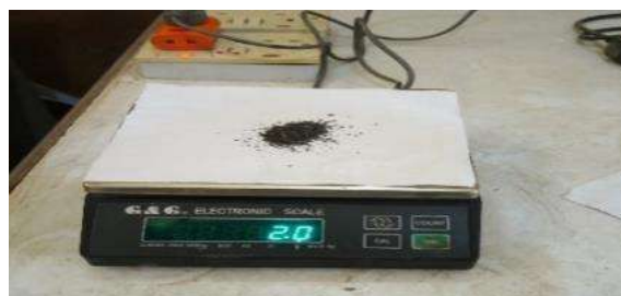
Figure 2: Electronic scale used for measuring cast iron chips for corrosion test.
