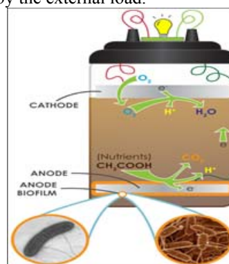
Figure 1. A diagram of a Soil-based MFC (Source: [23])
