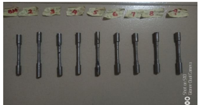
Figure 6: Extracted tensile specimens machined for the Test.
