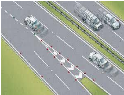
An edge line which slants towards the centre of the road forewarns that the road is narrowed ahead
