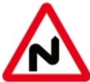
DANGEROUS DOUBLE BEND (FIRST TO RIGHT)
