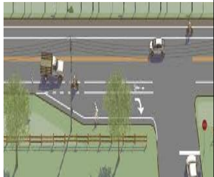
An edge line crossed only by traffic moving to and from the shoulder of the road.
