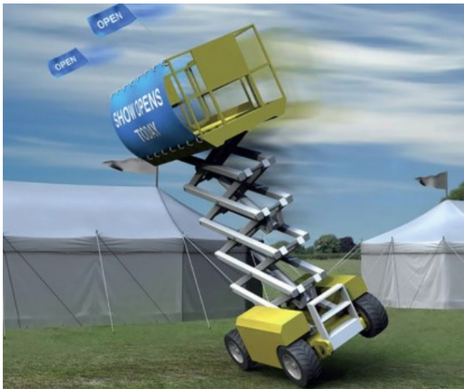
Figure 1: Effect of wind on mobile Scissor lifting system [5].
