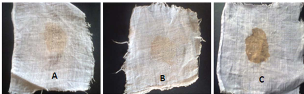
Figure 7. Destaining of blood-stained cloth by crude keratinases. Note: Destaining blood by the wild-type strain after 3 h of incubation (A), by the mutant strain after 2 h of incubation (B) vs. a control (C) incubated in water.
