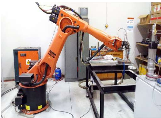
Fig. 3. The laser system used in depositing the composite coating.
