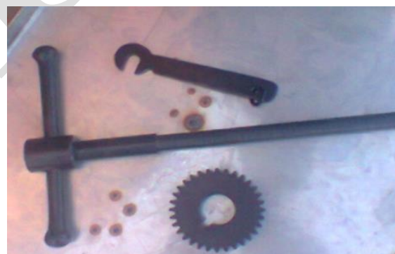
Figure 4: The parts after Parkerizing.
