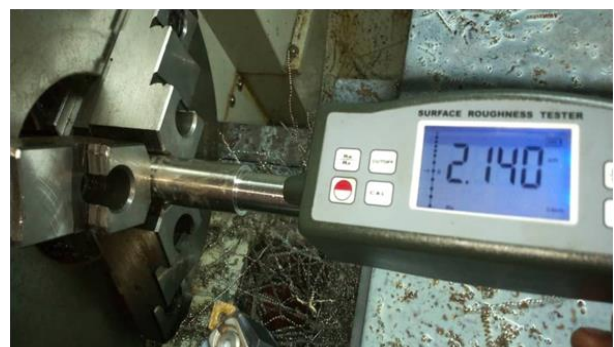
Plate III: Set up for measurement of surface roughness of turned surface.
