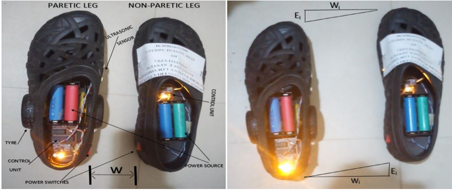
Fig. 7. A design prototype for the robotic wearable shoe.
