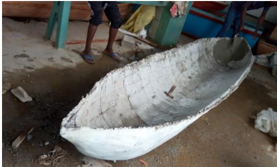
Plate 1: Cured canoe hull removed from the mould
