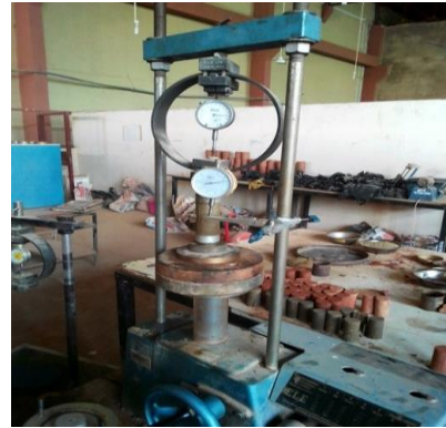
Figure 2 Unconfined compressive strength test
