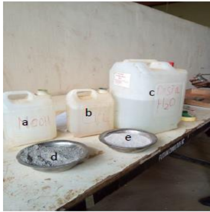
Figure 1 Additives used: a) sodium hydroxide, b) calcium chloride, c) distilled water, d) cement, e) RHA
