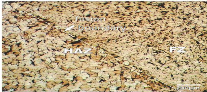
Fig.10: Microstructure of weldment from experimental run 8
