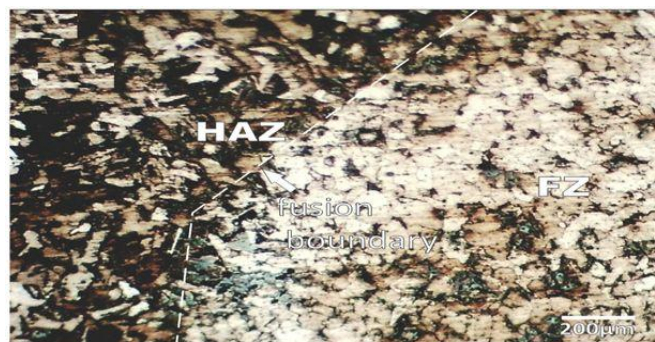
Fig.8: Microstructure of weldment from experimental run 6
