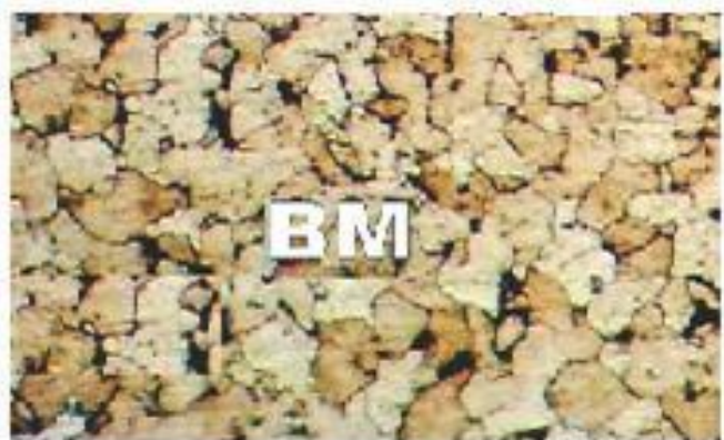
Fig. 2: Microstructure of base material
