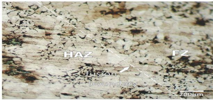
Fig.9: Microstructure of weldment from experimental run 7
