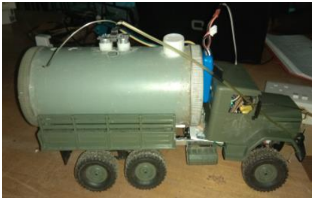
Fig. 6. Packaging of oil and gas automobile tanker tracking system prototype
