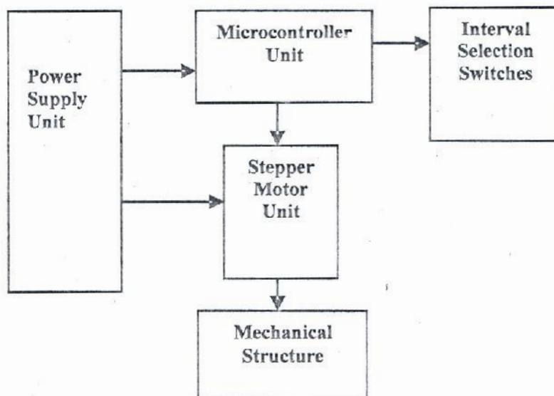
Fig 1: Block diagram of Automatic fish feeder
