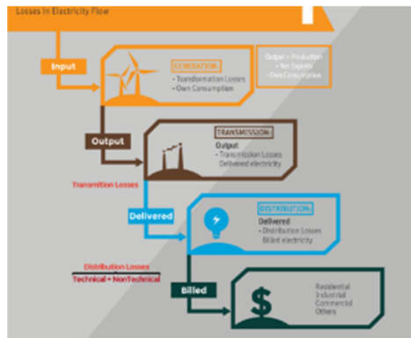
Source: Figure 1: Aggregated technical, commercial, and collection loss
