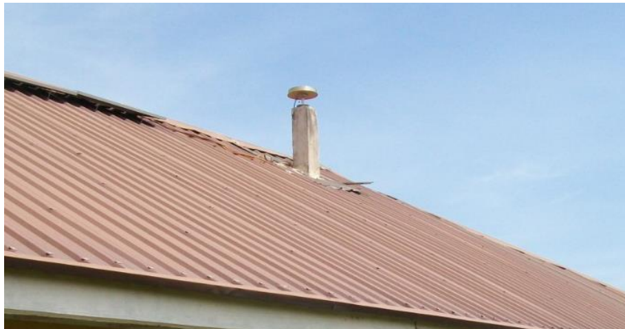
Plate 1: The CORS located on the roof of the Faculty of Environmental Technology building at Moddibo Adama University, Yola.
