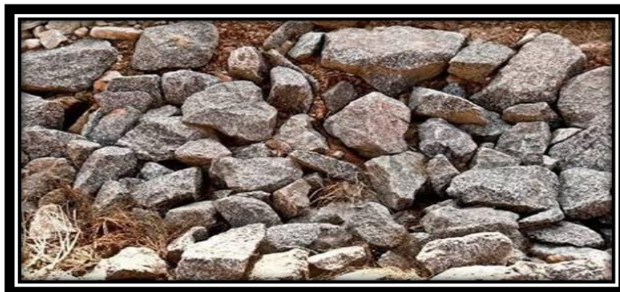
Plate 1: Shows granite stones used for construction. Source: Alao L.O (2021)
