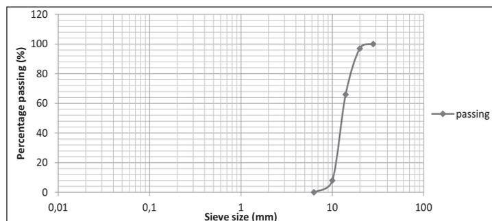
Figure 1. Particle size distribution of coarse aggregate
