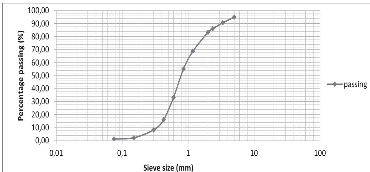
Figure 2. Particle size distribution of fine aggregate
