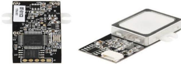
**Figure 7.** Rear & Perspective view of the GT511C3 Fingerprint Sensor (Adapted from "GT-511C3 Fingerprint scanner hardware, wiring and connector numbering" by Starting Electronics, 2014. Retrieved from <https://startingelectronics.org/articles/GT-511C3-fingerprint-scanner-hardware/>).
