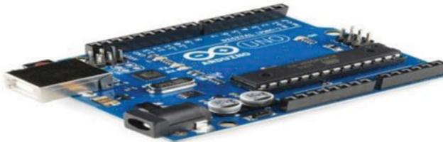
**Figure 6.** The Arduino Uno Board (Adapted from "Embedded system design with Arduino, 8051MCU and PIC16887F: A laboratory manual" by O. M. Olaniyi, F. Sado, O. Rabi, C. Inalegwu, & D. Maliki, 2013b, Department of Computer Engineering, Federal University of Technology, Minna, Niger State).
