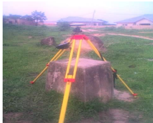
Figure 5 DGPS Set-Up at L40 Acquiring Satellite Data
