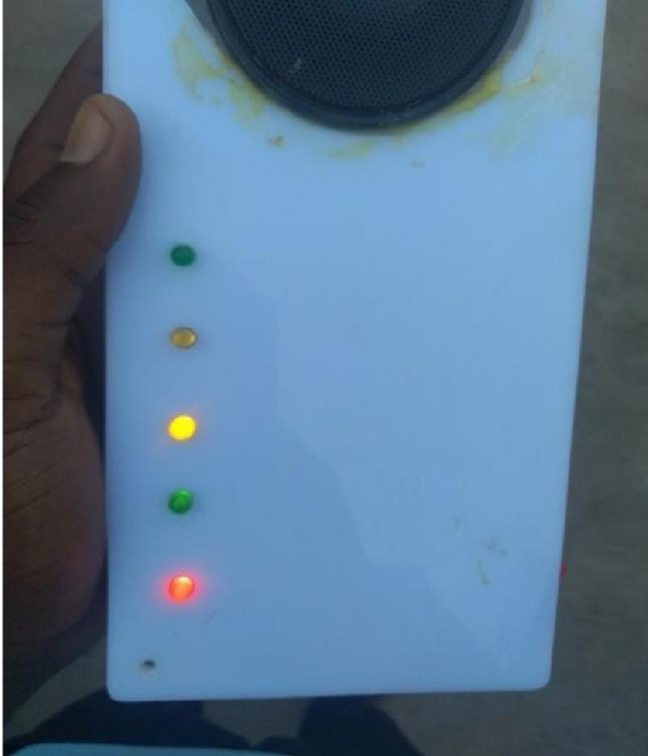
Figure 9: system indicating the bus has reached Kpankungu Roundabout
