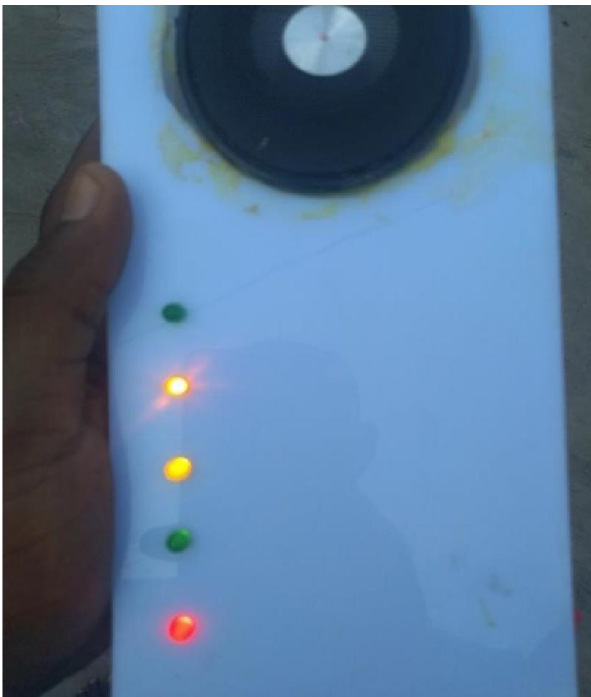
Figure 10: system indicating the bus has reached NECO Office
