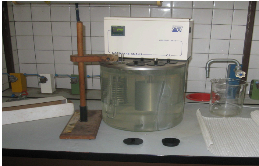
Plate 3: Experimental setup (Water bath and Viscometer)
