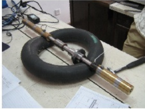
Figure 5.3 Rotor-only EMA test set-up
