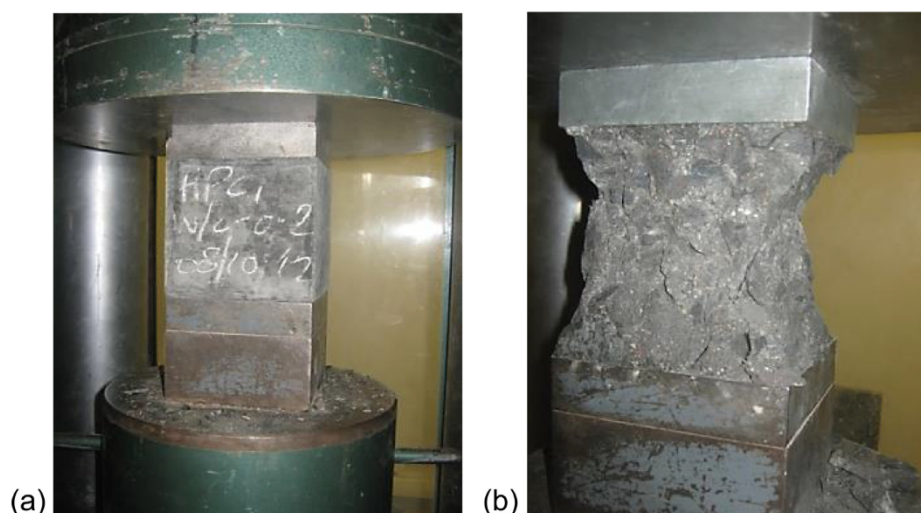
Fig. 1. Compressive strength test setup (a) before failure, (b) after failure.
