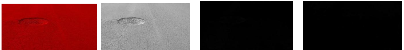
Figure 6: Original RGB image transform using YIQ colour space model
