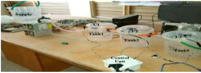
Figure 1: Automated multiple water tanks control and implementation
