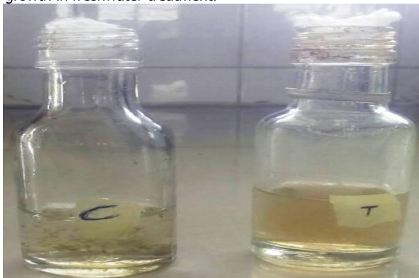
Fig. 7: Anticyanobacterial activity of AgNPs against a bloom forming cyanobacterial strain. C, profuse cyanobacterial growth in control experiment without AgNPs and T, inhibition of cyanobacterial growth by the synthesized AgNPs
