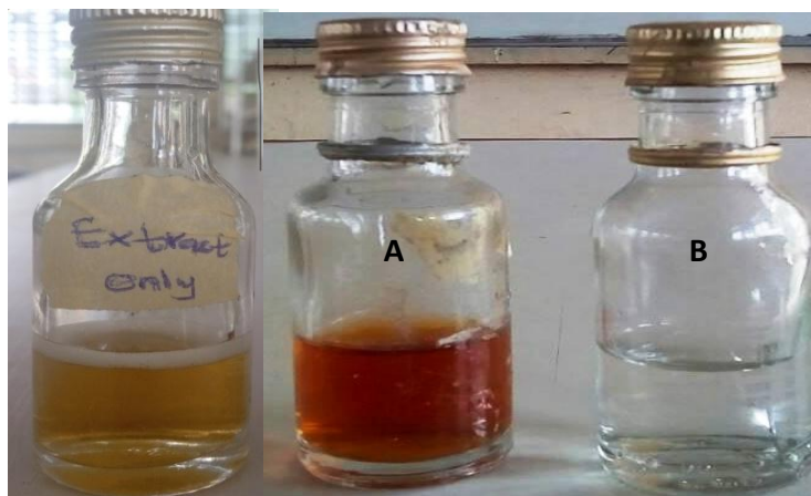
Fig. 2: Biosynthesized AgNPs using aqueous extract of ginger rhizome: A, synthesized AgNPs within 10 min; B, control silver nitrate solution
