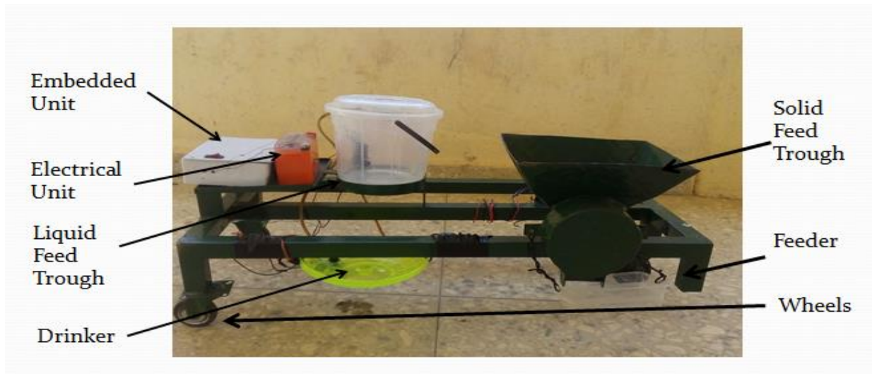
Figure 6: Overview of the developed mobile intelligent poultry feed dispensing system
